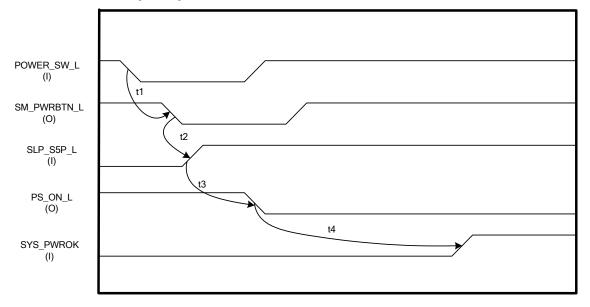
Figure 14. Typical Power-Up Sequence
